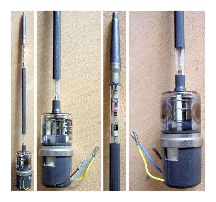
TWT amplifier. Frequency range: 5.85 to 7.2 GHz. 25W max saturated out power, 36 to 43 dB gain at 10W.
