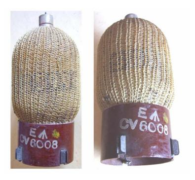
Spark gap 'trigatron' for delay line discharge/pulse forming.
