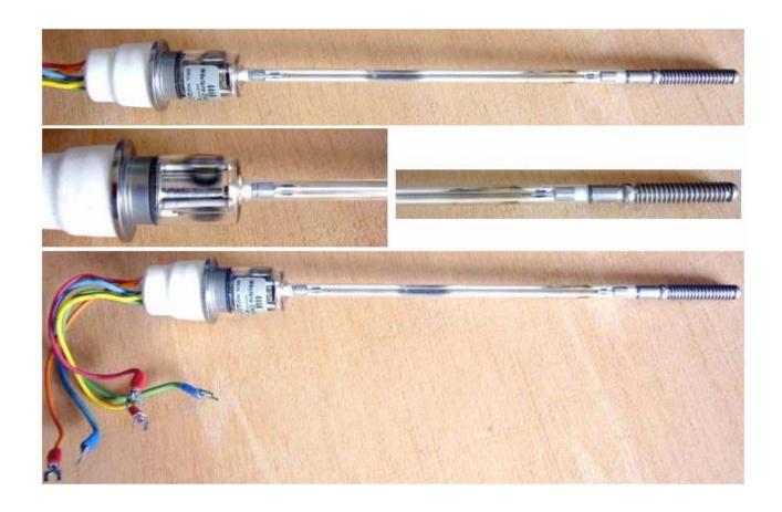
Western Electric TWT amplifier, external waveguide mounting and external focusing magnet. Heat radiator required at the collector.
