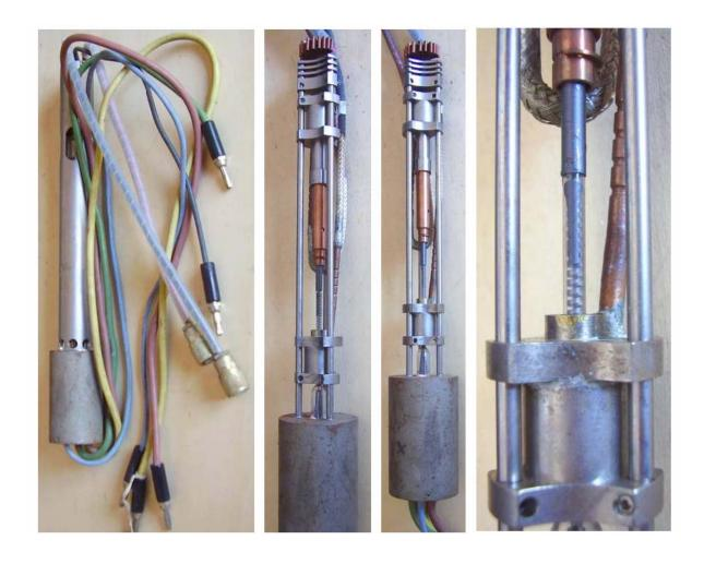
No information found about this TWT. TNC RF connectors. Probably used inside lab instrumentation, due to the presence of the banana plugs.
