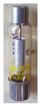
Argon-Hydrogen filled spark gap, intended for use as radar modulator. Scaled down 1B22, aluminum cathode with internal corona points to start the firing. Typically used in series pairs with triggering pulse applied to one of them. Must be operated with cathode aperture downward.
