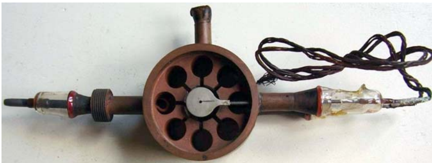
Fig.1 - E.1189 eight-slot prototype recently found. Believed to be the very early of the four samples listed by Megaw in his secret report and built at GEC in the Summer 1940. First operated around 30 July.
